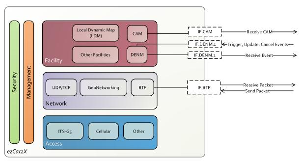
All logical interfaces are provided as ZeroMQ (e.g. via TCP) running on the same IP host in the subnet. The subnet address, host IP and port numbers of the interfaces are configurable.
