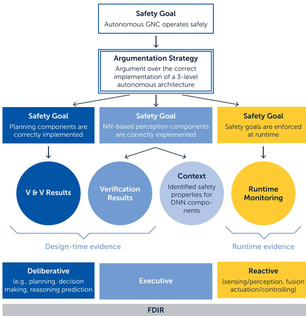
Figure 3. Safety case from a 3-layer architecture of a cognitive system.
